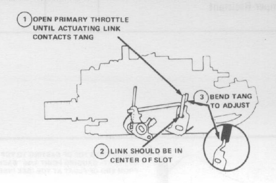
FIG. 14 SECONDARY OPENING ADJUSTMENT
