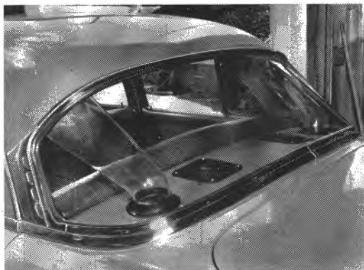
FIG. 5—Plastic discharge outlets are used by Novi to direct flow of air forward along roof of car.
