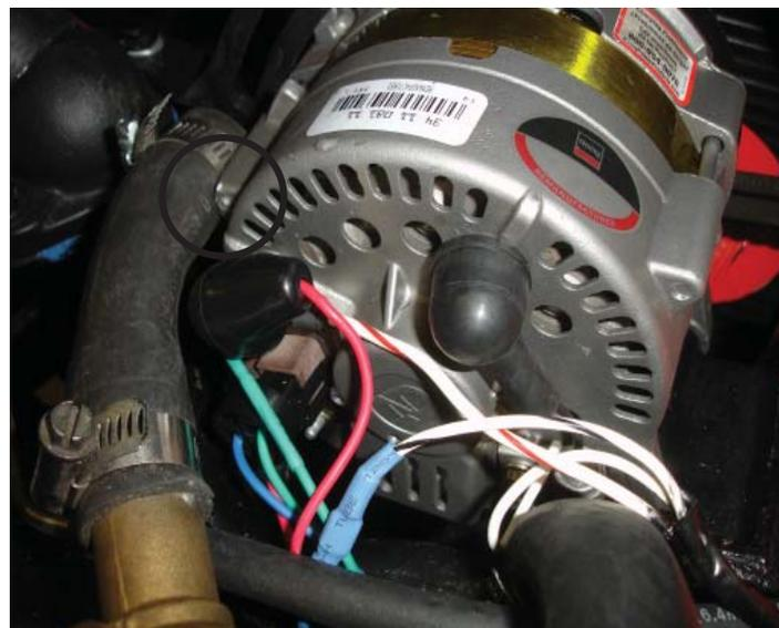
Run a simple jumper wire from the BAT terminal on the back of the alternator to the S blade terminal. The "IG" terminal needs a wire connected to it that is hot with the key turned to the ON position. Moving the white with black stripe wire from the FLD connector to the IGN lug on the voltage regulator will provide that.
