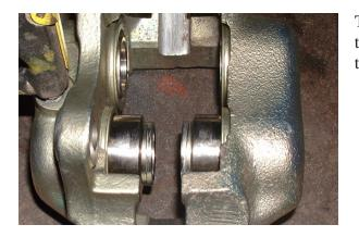
This is the whole caliper before taking it apart. Note the air-gun nozzle feeding air into the lower port on the far left to blow the pistons out.
