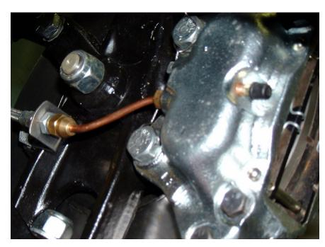
This method enables a single line connection for the fluid to the caliper. I think this is much neater.
