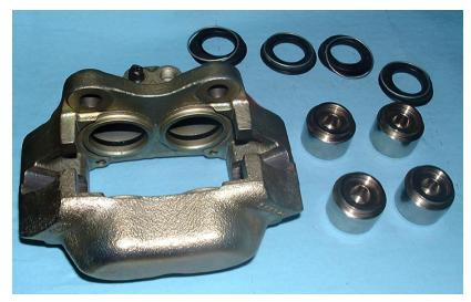
And here is what it looks like after splitting the halves. Note the sealing "O" rings on the lower half.
