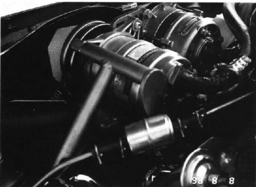
Closeup view of bracket with compressor installed
