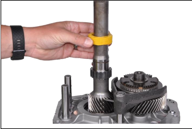
8.29: Install mechanical speedometer gear with detent ball to main shaft (Note: Ford=12 tooth; GM=17 tooth)
