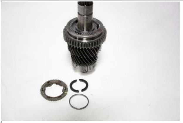
5.8: Remove 1 st gear locking ring split washers and blocking rings
