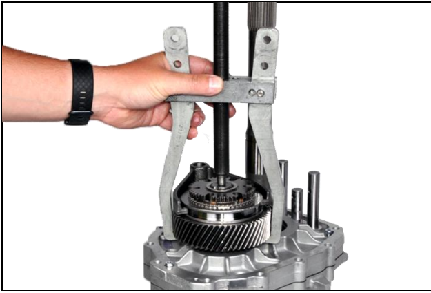
3.20: Using a two-jaw puller, remove 5 th gear and synchronizer assembly
