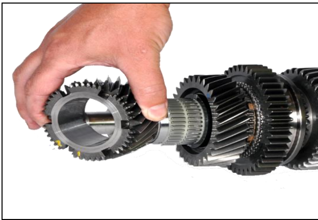
5.10: Remove 3 rd gear from Main shaft.
