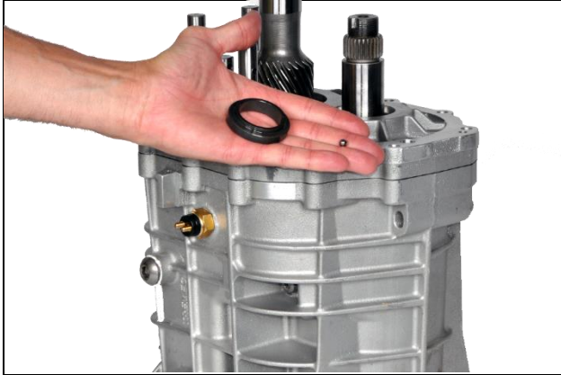
8.22: Install 5 th gear bearing and thrust washer to cluster shaft
