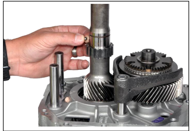
3.16: Remove steel locking ball
