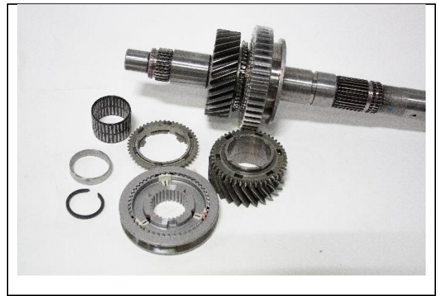
5.11: Remove 3 rd gear bearing thrust washer 5.12: Remove 3 rd gear snap ring and blocking rings.
