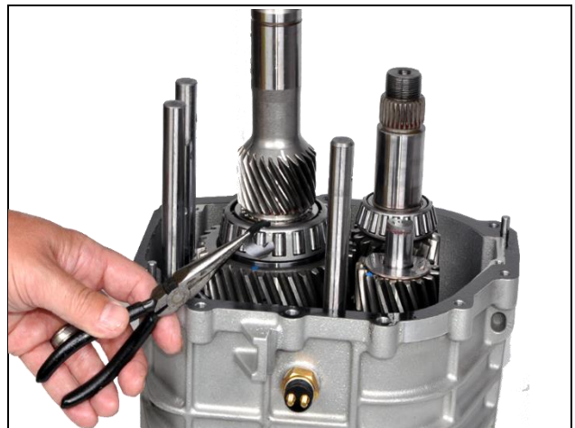
3.26: Remove snap ring from 5 th reverse selector link inside main case
