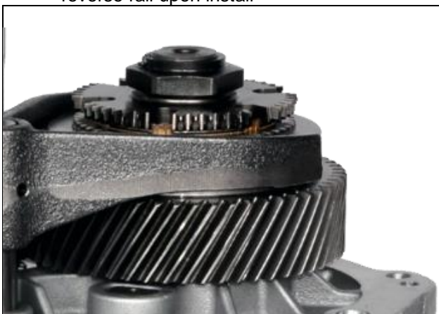
8.27: Install counter shaft locking nut. Torque nut to 100 ft/lb (Stake nut to shaft)
