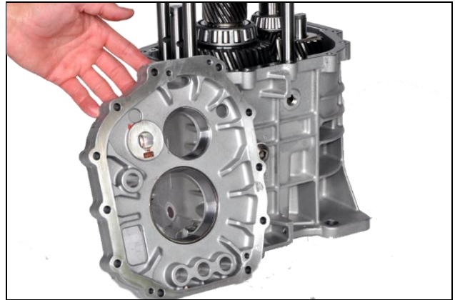
8.10: rotate transmission onto its face and remove intermediate plate.
