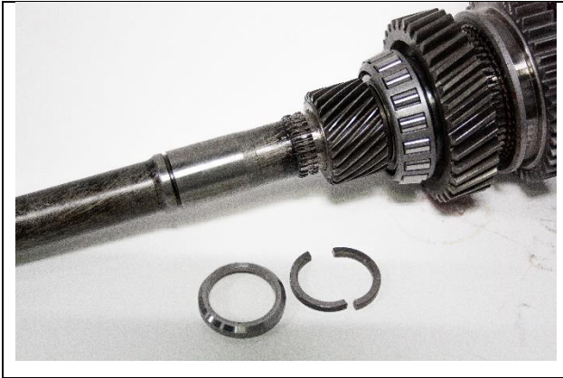
5.1: Remove 5 th gear lock ring and two-piece snap ring from Main shaft
