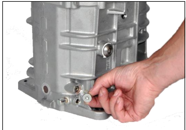
8.14: Install detent plunger spring and nut on either side of main case. Torque to 15-25 lb-ft
