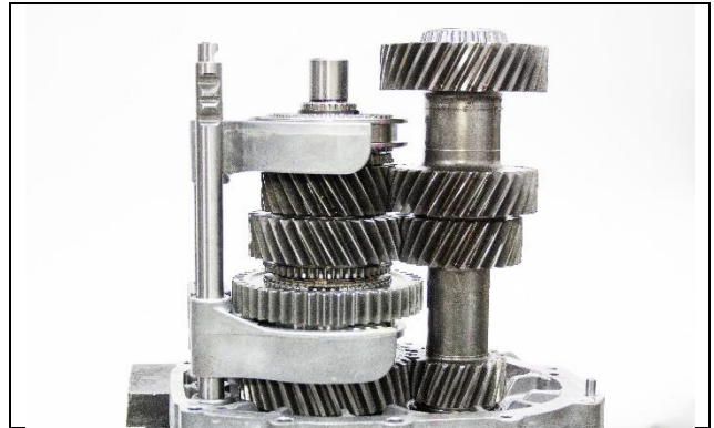
8.3 Install Counter shaft assembly into midplate
