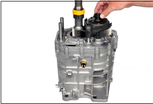
3.12: Position transmission in vertical position to access rear.
