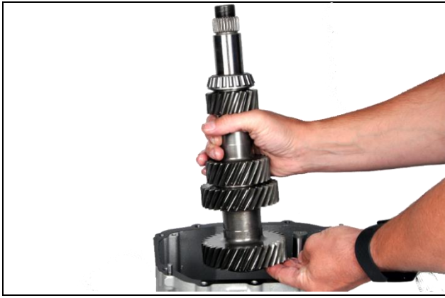
3.36: Remove cluster shaft from case
