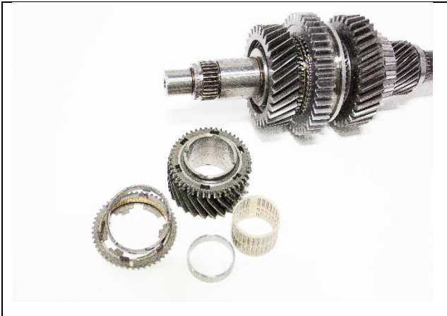
6.13: Install 3 rd gear bearing onto main shaft
