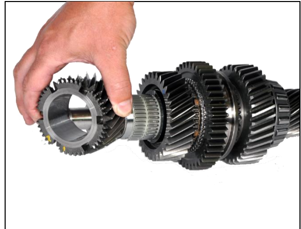
6.14: Install 3 rd gear and blocking ring
