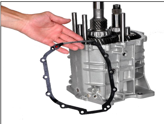
3.25: Remove extension housing gasket
