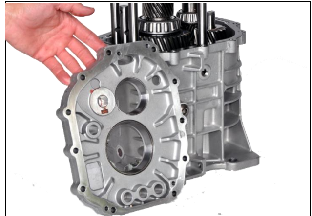
8.18: Install rear housing gasket and intermediate plate. (Note: Be careful to line up idler gear thrust washer.)
