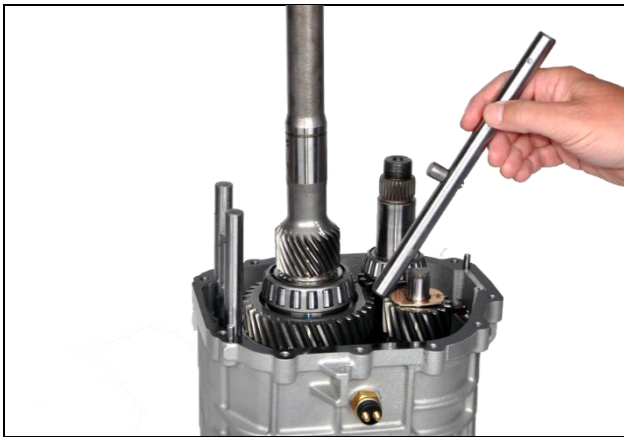
3.27: Rotate 5 th reverse shift rail counter clockwise and remove from case
