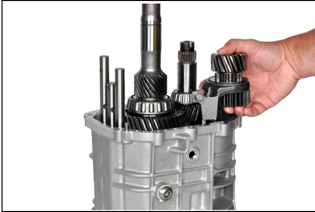
8.15: Install reverse idler synchronizer and fork into case
