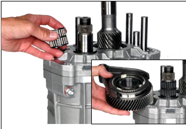
8.24: Install 5 th gear bearing to cluster shaft
