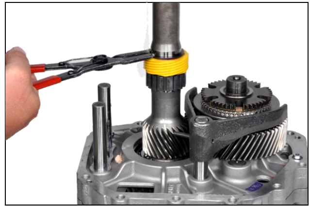
3.14: Remove speedometer gear snap ring
