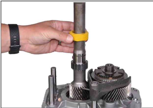
3.15: Remove mechanical speedometer gear
