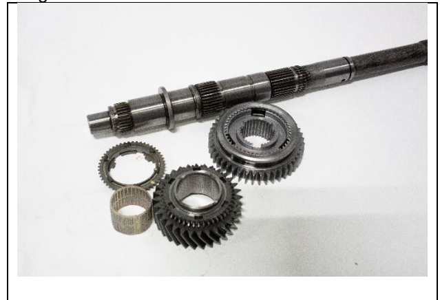
5.14: Remove 2 nd gear bearing and blocking rings
