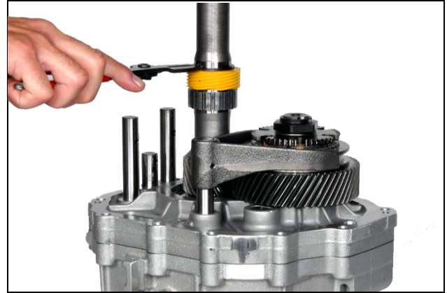
8.30: Install speedometer gear snap ring
