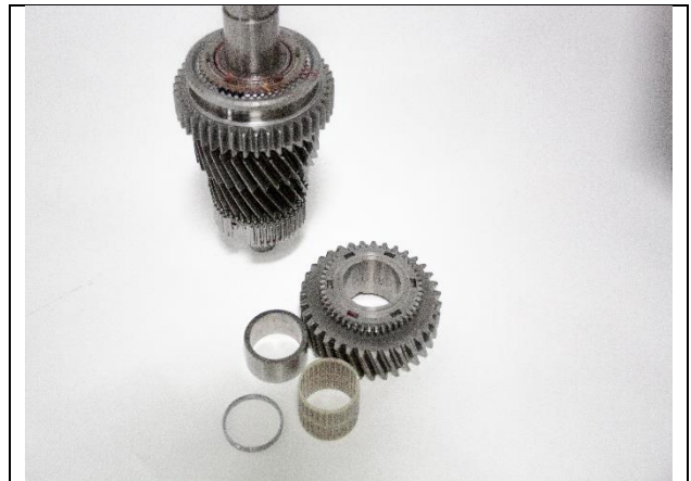
5.6: Remove 1 st gear from main shaft 5.7: Remove 1 st gear bearing, thrust washer and bearing journal from main shaft.
