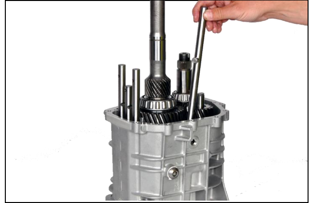
8.16: Install 5 th reverse shift rail into case (Note: Rail detent roller fits in selector arm)
