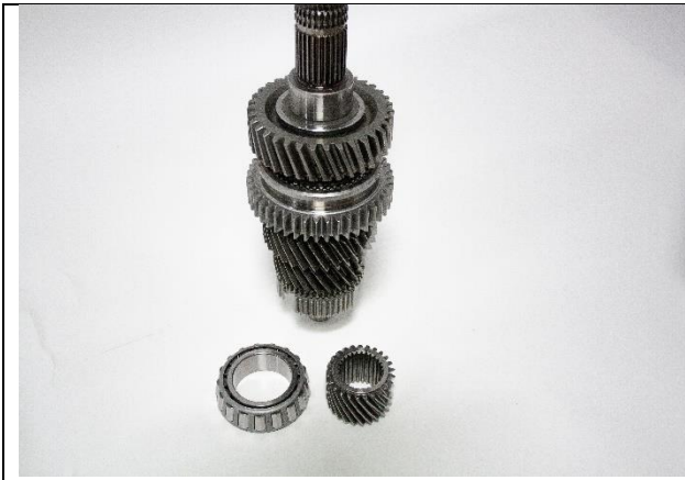
5.3: Remove 5 th drive gear and bearing from Main shaft.
