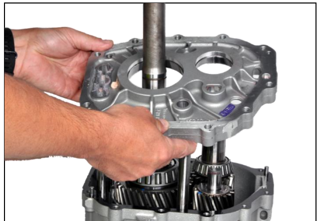
3.24: Remove mid-plate from main case
