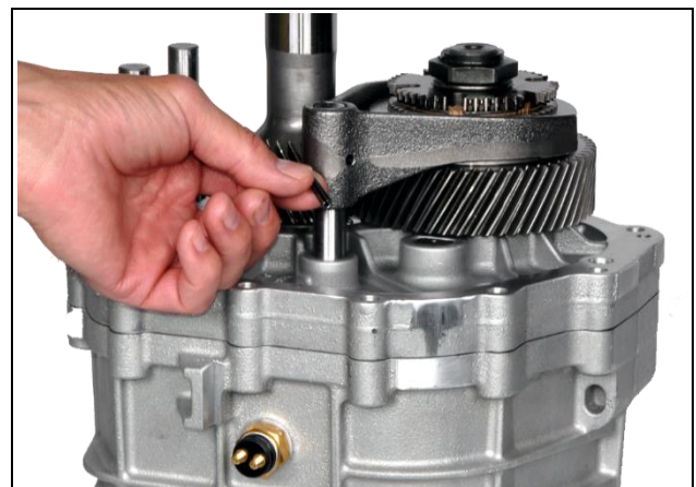
8.28: Install 5 th reverse fork roll pin to rail
