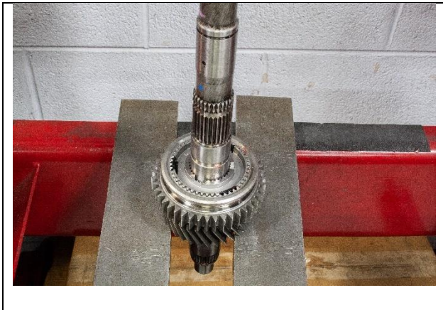
5.13: Using a press remove 2 nd gear and 1-2 synchronizer
