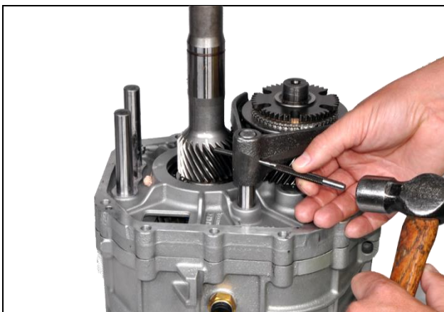
3.17: Remove 5 th gear fork roll pin
