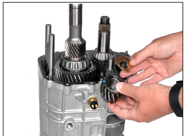
3.30: Remove reverse idler gears and synchronizer from case
