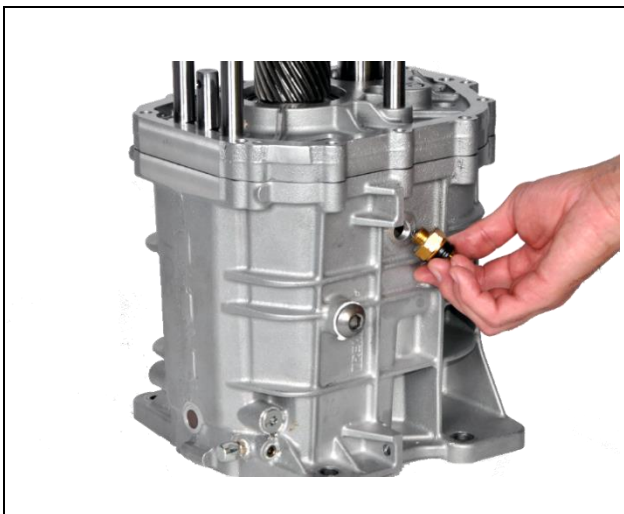
8.19: Install reverse light switch in case. Torque to 12-16 lb-ft
