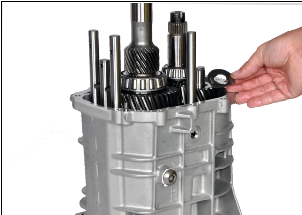
8.17: Install reverse gear thrust washer on top of idler gear (Note: Place tab in the 12 o'clock position)
