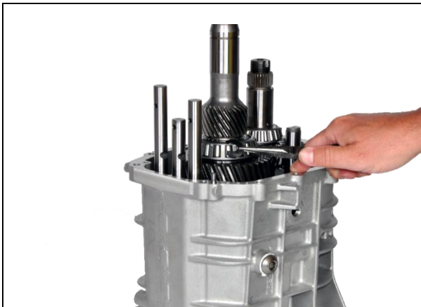
8.13: Install pivot pin snap ring
