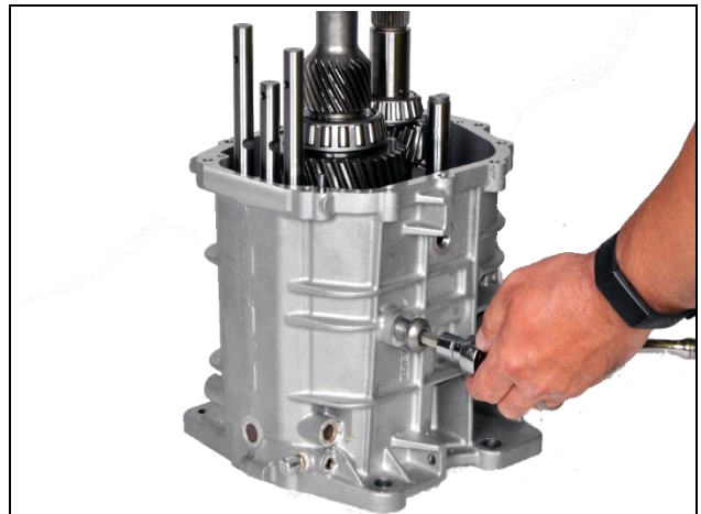
8.12: Install 5 th rev pivot pin bolt into case
