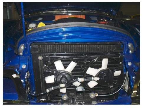
The condenser was mounted in front of the radiator with two auxiliary fans in front of that.
