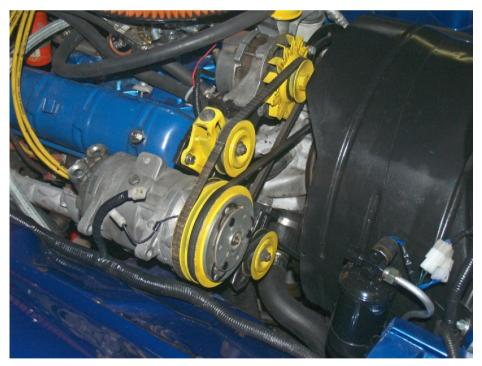
Here you can see the drive belt in place and the receiver drier mounted on the front radiator support.
