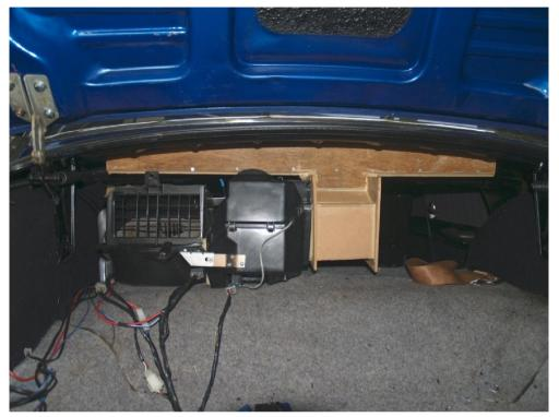
The fan, evaporator and wiring mounted to the air duct.
