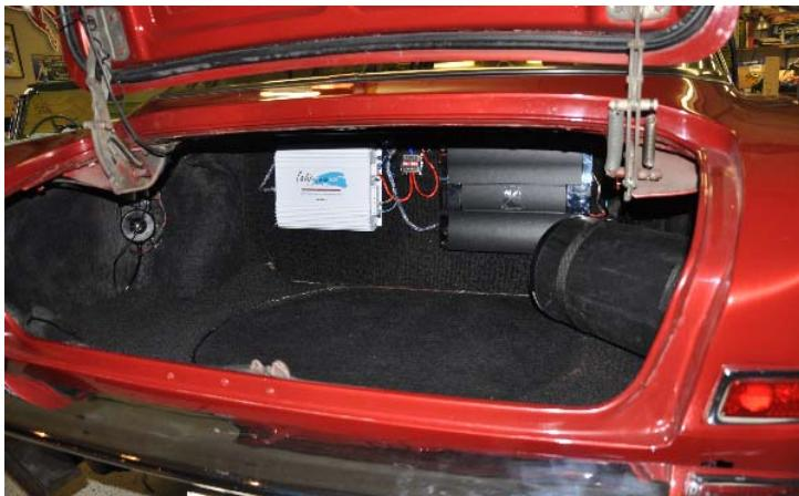
In steel bodied cars, external amplifiers are mounted on wood to prevent an undesirable condition known as "ground loop", and then the wood is screwed to the steel car body. While this is not truly necessary on a fiberglass car like the Avanti, I cut a  $\frac{1}{4}$ " plywood panel exactly the size of the panel behind the gas tank, and screwed the amps and power connectors to this panel, after gluing more of our carpeting to the panel. I then
