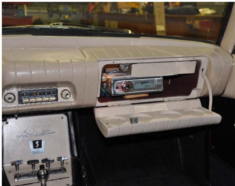
The head unit fits tightly inside the glove box, sitting on a four inch square  $\frac{1}{2}$ " piece of wood; everything is secured in place with Velcro. (Below) Using a 1" hole saw I bored a hole in the back left corner of the glove box for all the wires to pass through. I suggest removing the felt liner before cutting the hole and gluing the liner back afterwards. In use,
