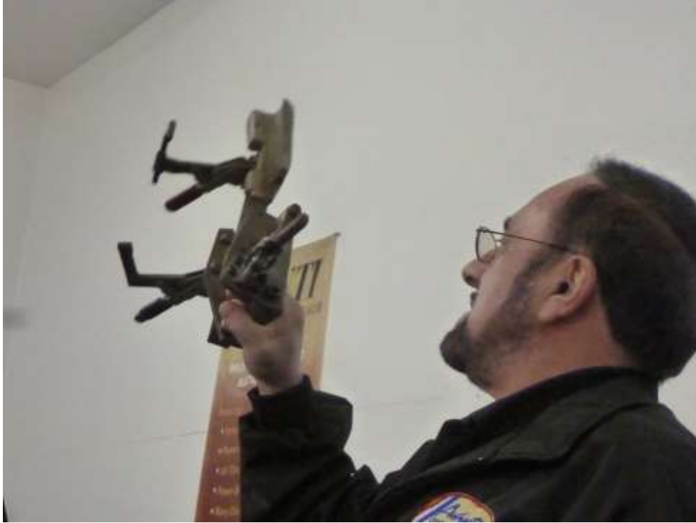
Editor Al holds up a piece of Studebaker Avanti memorabilia from his collection – One of the many 53 year old clamps that were used in the Studebaker Avanti Factory to bond the fiberglass body pieces together. You can see them hanging from the ceiling in the factory photo shown below
