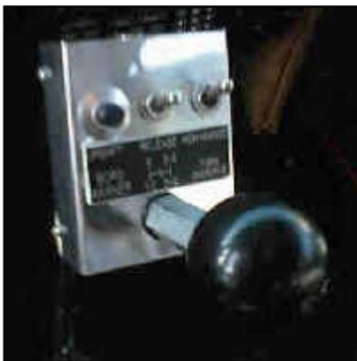
This is the split-shift control box in my 'Burb. The left button is SHIFT-UP, the middle is RELEASE, and the right is HIGH-RANGE. The engaged indicator is on the dashboard. I added rubber grommets to isolate it from the gearshift shaft to eliminate transmission noise from the cab.
