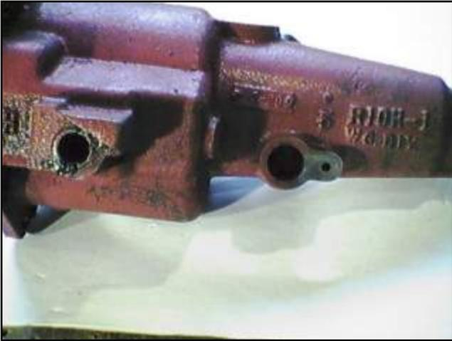
This is a Borg Warner T-85N case with the components removed. The hole on the left is for the freewheel clutch lockout. The right hole is for the speedometer. These photos are of my spare overdrive unit.
