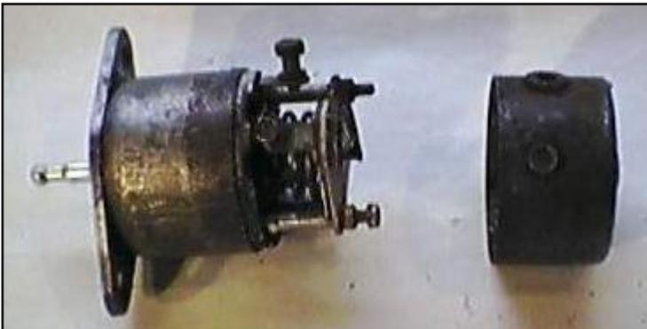
The overdrive solenoid with the cover removed. When powered, the shaft puts pressure on locking dogs until engine torque is released, then the locking dogs engage the planet set case, and the ring gear then rotates 27% faster than the input shaft. The large terminal is the (S)olenoid line, and the (I)gnition terminal has a short to ground when the shaft is in the engaged position.
