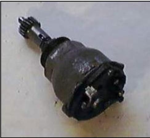
This centrifugal switch (Borg Warner calls it a governor) is a key part of the O/D setup. It switches to ground at 27 MPH, and releases at 21 MPH. They put thought into the speeds at which it operates. If you are in 2nd, it will shift up at 27 MPH. You let up on the gas, then step on it again for 2nd over. When you turn a corner, it will automatically downshift back to 2nd as you make the turn. It's GREAT!!
