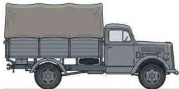
OPEL BLITZ (GERMANY) | Drive: 4x2 (Rear Wheel Drive) Cargo: 3 Tons | Terrain: Roads Only
