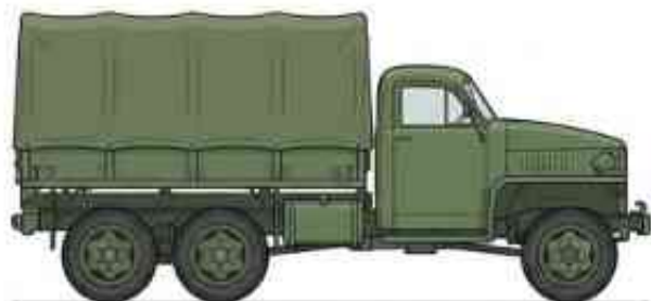
STUDEBAKER US6 (USA) | Drive: 6x6 (All Wheel Drive) Cargo: 2.5 Tons | Terrain: Mud & Snow
