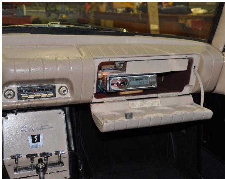
The head unit fits tightly inside the glove box, sitting on a four inch square 1/2" piece of wood; everything is secured in place with Velcro. (Below) Using a 1" hole saw I bored a hole in the back left corner of the glove box for all the wires to pass through. I suggest removing the felt liner before cutting the hole and gluing the liner back afterwards. In use,
