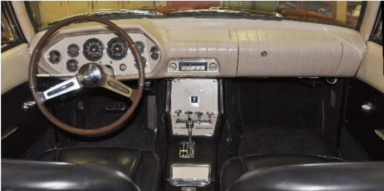
➤ Before...or after? You can't tell, and that's exactly the point. This is an “after” shot. Head unit hidden in the glove box; speakers out of sight under the dash; controls under the lid of the center console; and amplifiers in the trunk.
