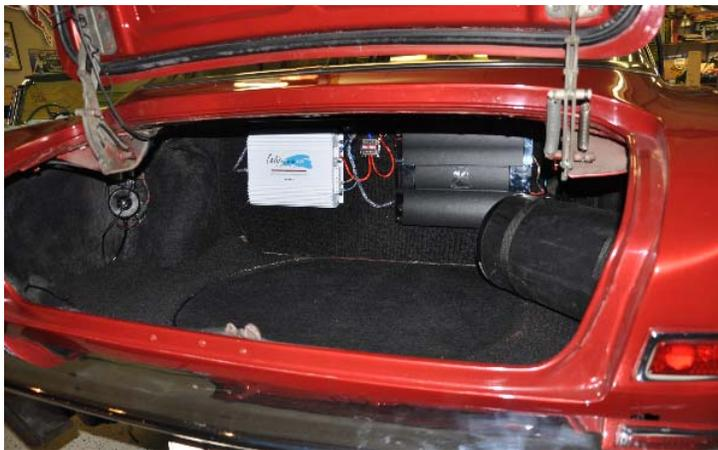
In steel bodied cars, external amplifiers are mounted on wood to prevent an undesirable condition known as "ground loop", and then the wood is screwed to the steel car body. While this is not truly necessary on a fiberglass car like the Avanti, I cut a 1/4" plywood panel exactly the size of the panel behind the gas tank, and screwed the amps and power connectors to this panel, after gluing more of our carpeting to the panel. I then
