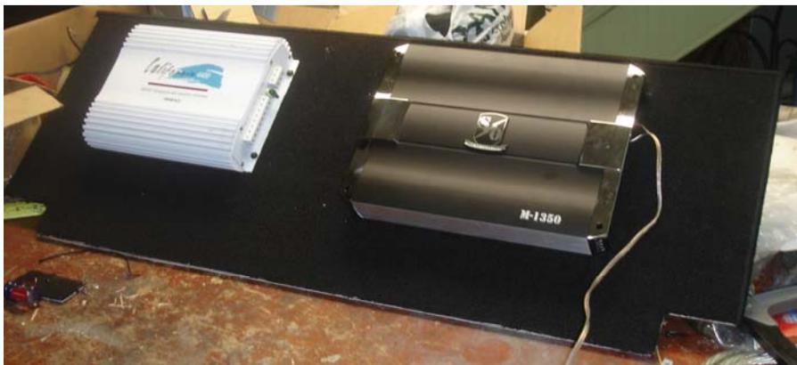
My installation uses two external amplifiers. One is a mono amplifier specifically dedicated to the subwoofer. The other two channel stereo amp powers the front component speakers (separate woofers and tweeters). The amplifier
