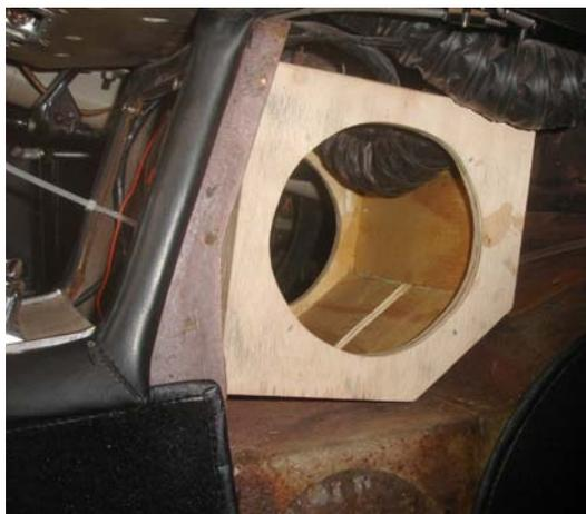
These photos show the basic construction of the speaker box using 3/8 plywood. Notice that the speakers are separated from each other by a solid wooden baffle inside the case. The box is
