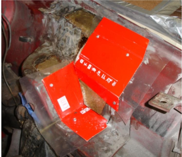
The key is to work from the back, creating a mold on **top** of the damaged area and working to lay up the new fiberglass from the inside of the inside of the fender. I started with one single large flat surface, and created a mold using cardboard from a shoebox and used sheet metal screws to hold it in place.
