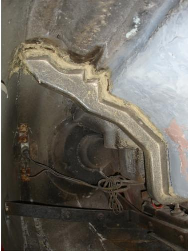
headed rivets that are appropriate for joining two thicknesses of fiberglass together. This brace is much needed to stiffen the battery box, and since it also keeps the panel from flexing when the hood is opened to its limits.
