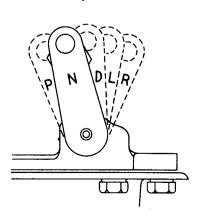
Park range. Then move the selector valve lever back one detent. In this position the selector valve lever will be in direct line with the forward band adjusting screw located immediately behind it on the transmission. (See opposite.) with the selector
