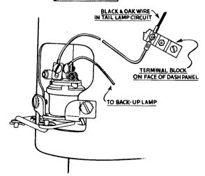
BRACKET AND SWITCH FURNISHED WITH KIT SHOULD BE DISCARDED WHEN MAKING THIS INSTALLATION.
