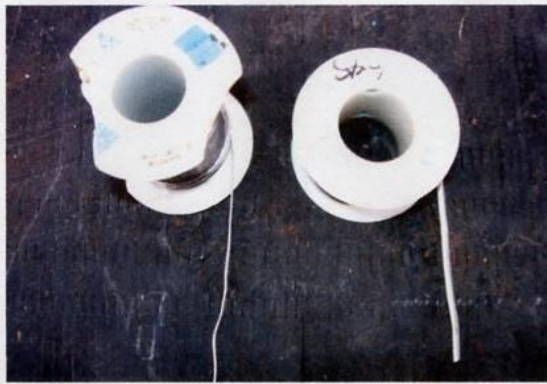
Solder: Left roll is solder for wires. Right roll is solder for plumbing. Do not use solder with acid core
