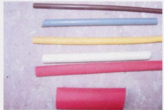
Heat Shrink Tubing: Used for insulation over the soldered connections. It is superior to electrical tape. Available in variety of colors, sizes and shrink values. Most will shrink to half size.
