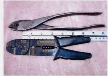
Crimpers: Top one- Industrial crimper preferred. Provides more leverage and better crimp.
