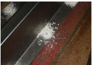
**Step 1:** Remove the seat, pull back the carpeting and peel off the glued-on vinyl that covers the floor at the seat's front mounting points. Judicious use of a heat gun may help soften the old adhesive, but be careful not to apply too much heat. If the bolts just spin in their holes, use vice grips from
