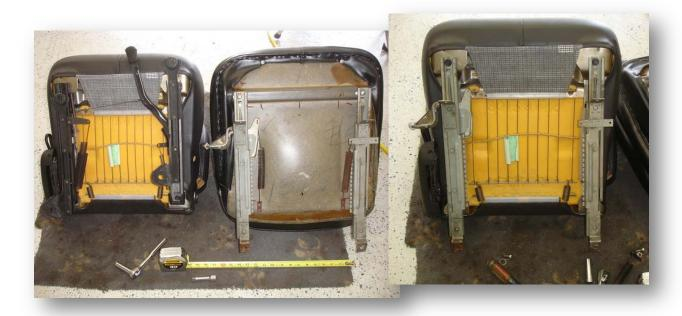
To my delight, I found that my Camaro seat front mounting holes line up nearly perfectly with the holes in the Studebaker tracks. However the back holes are then misaligned and leave a gap of about 1 ½ ". The simple solution is to make small adapter brackets to bridge the seat tracks to the seats' holes.
