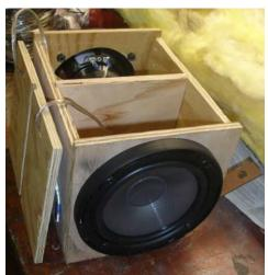
bolted to the transmission hump with two sturdy L-brackets. It fit tightly enough that I did not need additional points of connection, but I tested carefully by applying very loud music and listening for undesirable vibrations before I buttoned everything up.
