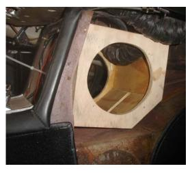
These photos show the basic construction of the speaker box using 3/8 plywood. Notice that the speakers are separated from each other by a solid wooden baffle inside the case. The box is
