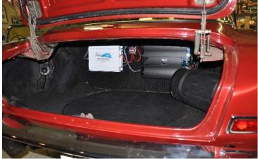
In steel bodied cars, external amplifiers are mounted on wood to prevent an undesirable condition known as "ground loop", and then the wood is screwed to the steel car body. While this is not truly necessary on a fiberglass car like the Avanti, I cut a ¼" plywood panel exactly the size of the panel behind the gas tank, and screwed the amps and power connectors to this panel, after gluing more of our carpeting to the panel. I then
